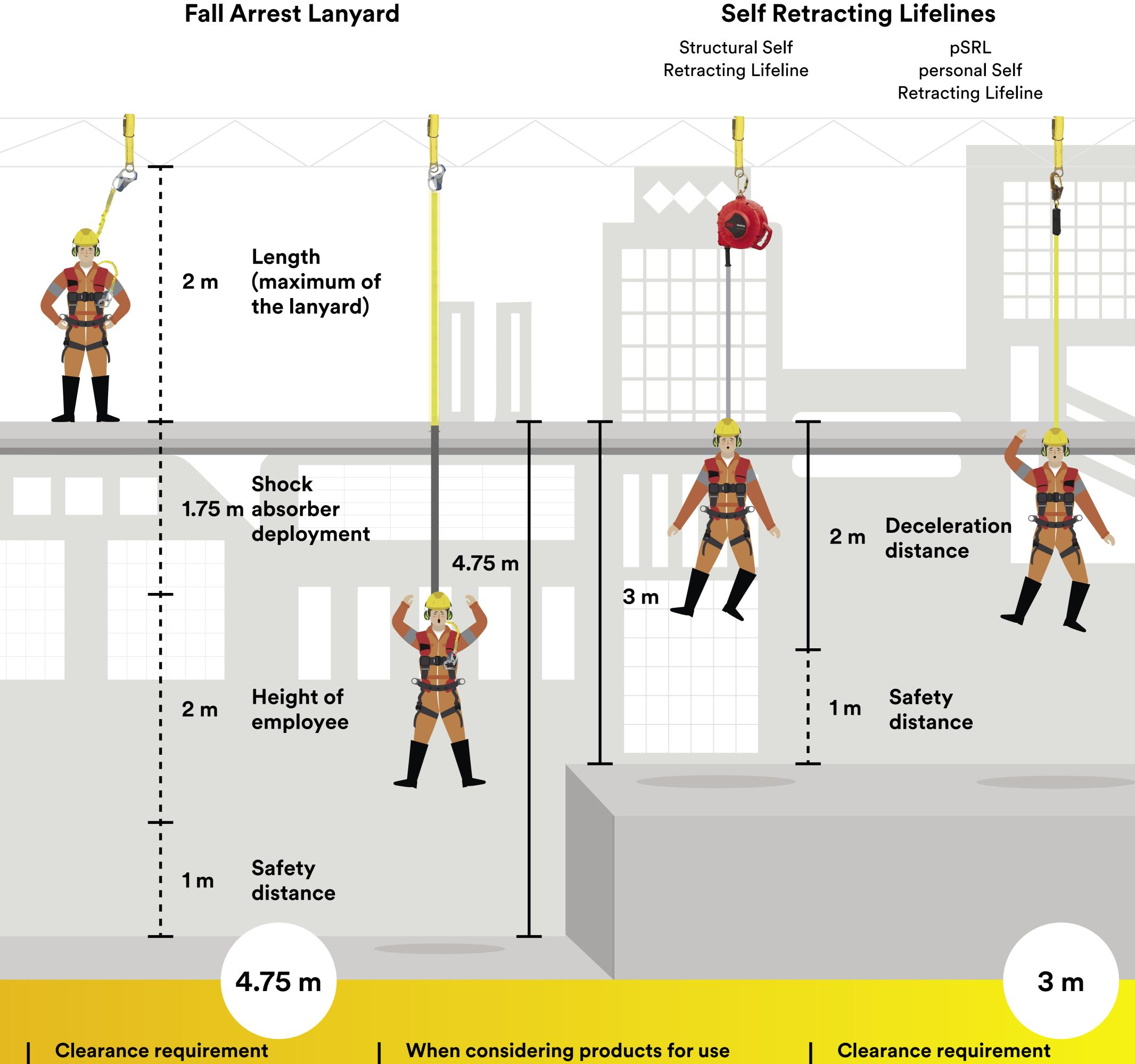
Clearance requirement from the work surface for a Fall Arrest Lanyard.\*
